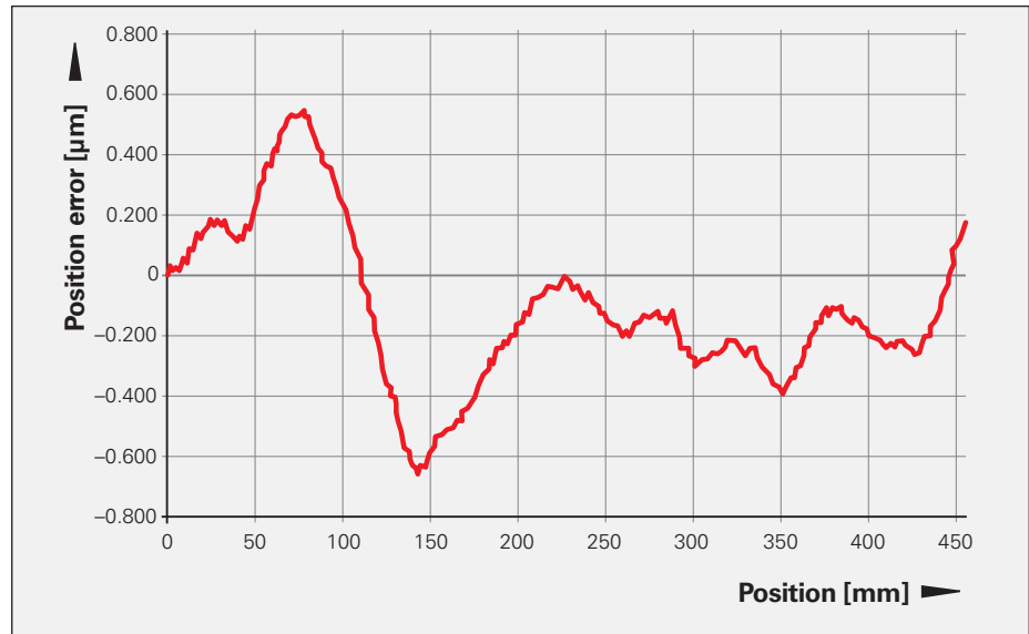
Figure 1: Typical position error over measuring length
