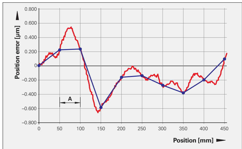
Figure 2: Compensation points for multipoint linear error compensation
