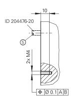
$\ensuremath{\mathbb{M}}$  = Measuring point for operating temperature/vibration
